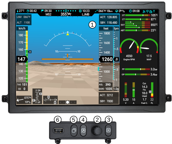
Figure 2.1: Nesis IV 10” display organization. A separate command panel named Kliki is connected to Nesis. Kliki is mounted separately from Nesis in any orientation.
