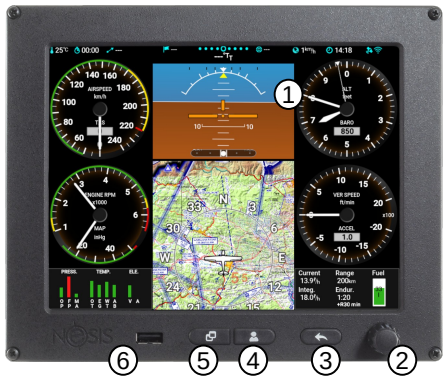
Figure 2.2: Nesis III display organization. Buttons and knob are integrated into the bezel.
