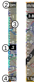
Figure 2.35: Illustration of vertical speed indication. Left is scale in ft/min right is scale in m/s.
