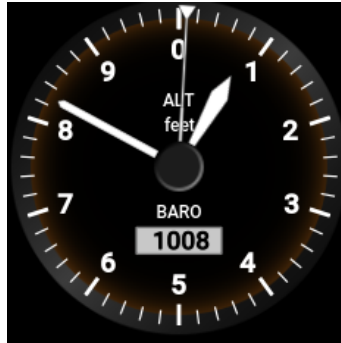
Figure 2.10: The altitude indicator with the scale given in feet. Three needles are shown in this case.
