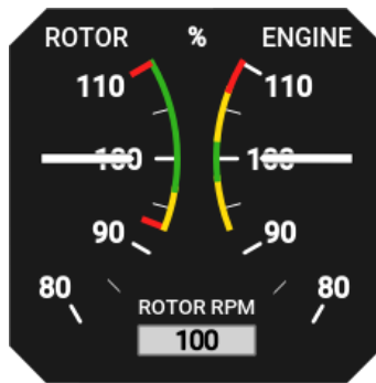
Figure 2.13: The combination of rotor RPM and engine RPM. Both scales are in percentages.
