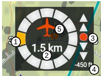
Figure 5.2: Threat classified as warning comes from left, distance is 1.5 km, about at the same visual level, 450 feet below.
