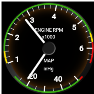
Figure 2.11: The combination of RPM and manifold pressure indicator.
