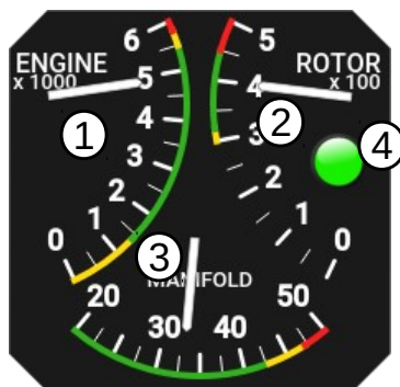
Figure 2.12: Four in one: the combination of engine RPM, rotor RPM, manifold pressure and prerotation helper lamp.
