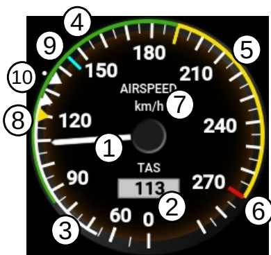
Figure 2.8: An airspeed indicator example optimized for an aeroplane using two step landing flaps.
