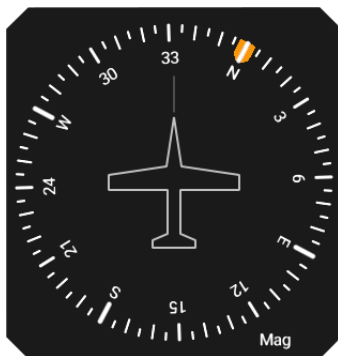
Figure 2.17: Illustration of the direction indicator.
