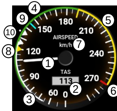
Figure 2.18: An airspeed indicator example optimized for an aeroplane using two step landing flaps.
