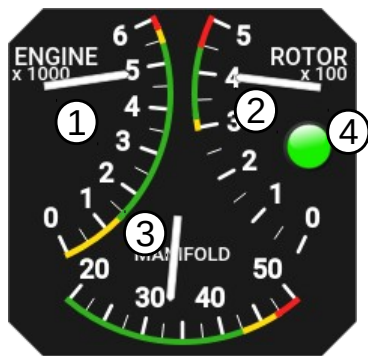
Figure 2.23: Four in one: the combination of engine RPM, rotor RPM, manifold pressure and prerotation helper lamp.
