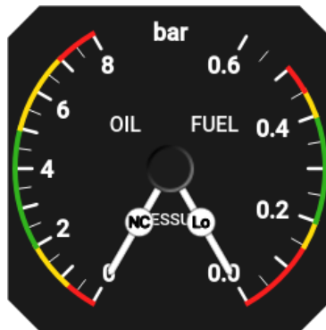
Figure 2.29: Round pressure indicator, with special markings shown on needles.
