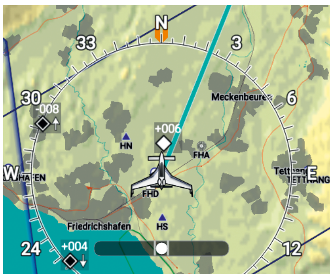
Figure 2.44: Traffic symbols on a map. Vertical difference is in hundreds of feet, as three digits are used.
