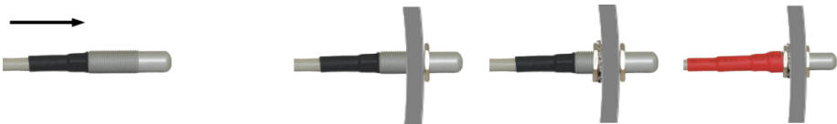
Figure 2.19: Inserting the OAT probe (left), cap is in place, tighten the internal nut, slide the insulation shrink sleeve (right).
