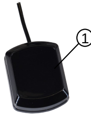
Figure 2.17: GNSS antenna orientation: ① – this side must face upwards, towards the sky.
