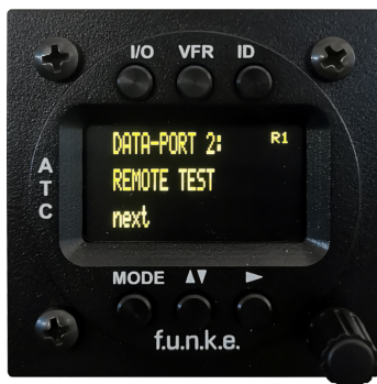
Figure A.6: Data-port 2 must be set to REMOTE TEST option.
