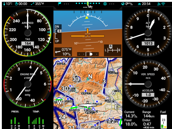
Figure 6.4: A typical example for automatically generated classic screen on 8.4" display.
