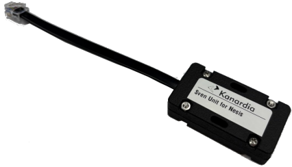
Figure A.1: Sven dongle for direct connection to Nesis. Note the RJ12 connector at the end of the cable.
