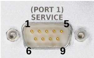
Figure 3.9: Service port D-SUB 9 male with designated pins.
