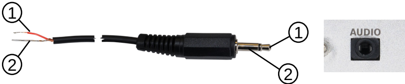
Figure 2.21: Audio cable: ① – audio signal, ② – GND
