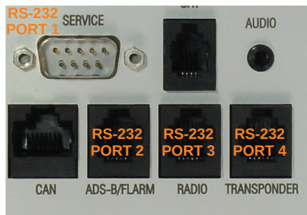
Figure 3.15: RS-232 ports at the back side of the Nesis.
