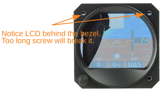
Figure 2: Example of broken LCD screen. Edge of the LCD display is visible behind the bezel.
