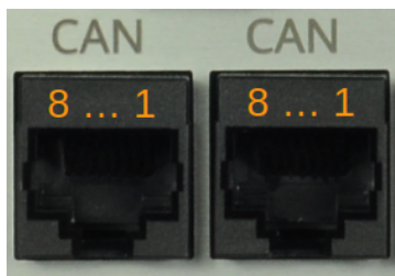
FIGURE 8 – Illustration du brochage des ports CAN.
