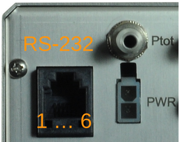
FIGURE 11 – Illustration du brochage du port RS-232.
