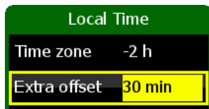
Figure 35: An example of local time set for Newfoundland and Labrador , which is UTC - 2h 30min.
