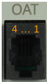
Figure 10: Pins of the OAT connector.
