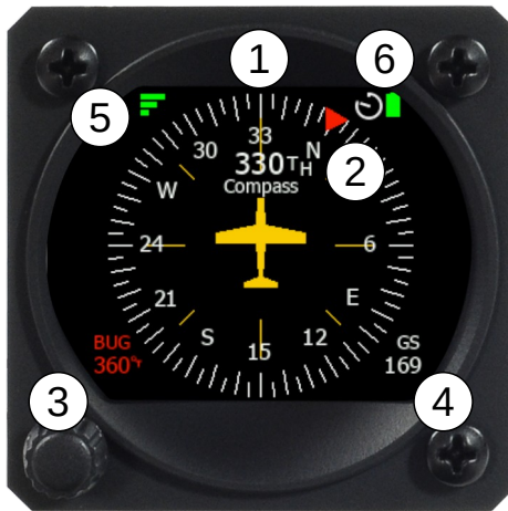
Figure 23: Direction Indicator screen with markings.
