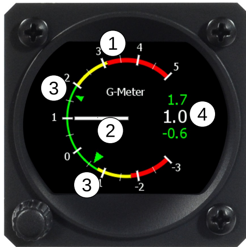
Figure 24: Horis G-Meter screen with markings.
