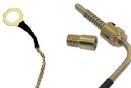
Figure 17: CHT ring terminal CHT probe (left), spring loaded bayonet type CHT probe with insert (right).
