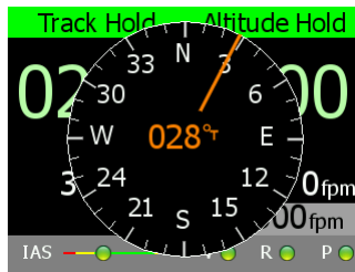
Figure 4: Navigation rose is shown for more intuitive track selection. Current track points upwards and orange needle points to a new track selection.
