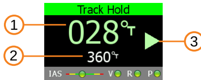
Figure 5: Upper part of the LCD display in the Track Hold mode.
