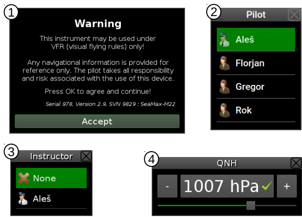
Figure 2: Typical start-up sequence.
