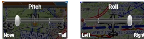
Figure 18: An example of the pitch trim and roll trim position window.
