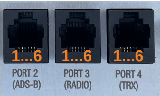
Figure 36: RS-232 ports with RJ12 connectors and their pin numbers.
