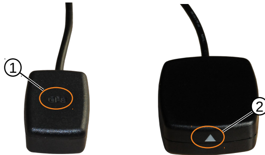
Figure 13: GNSS antenna orientation: ① – small, pure GPS antenna – the GPS text must be facing upwards, towards the sky. ② – larger combined GPS/Glonass antenna – the triangle must point upwards, towards the sky.
