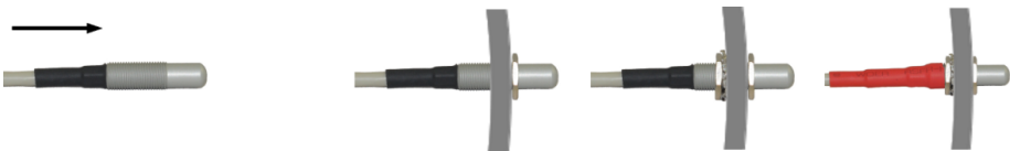
Figure 2.15: Inserting the OAT probe (left), cap is in place, tighten the internal nut, slide the insulation shrink sleeve (right).
