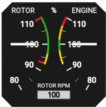
Figure 2.24: The combination of rotor RPM and engine RPM. Both scales are in percentages.
