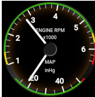
Figure 2.22: The combination of RPM and manifold pressure indicator.
